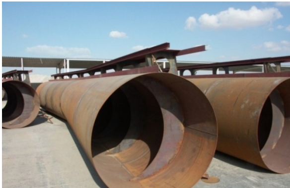
Figure 6: Steel torus elements
